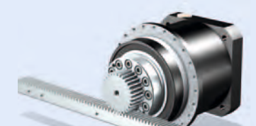
ZTR-PH(A), PHV(A) Rack and Pinion Drive Module 2 – 8 Feed force: 5.5 – 56 kN Feed velocity: to 4.7 m/s Helical and spur gearing
