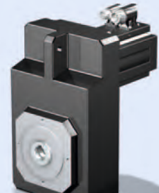
SMS F Offset Helical Geared Motor Acceleration torque: 19 – 1 100 Nm Backlash: Reduziert \leq 5 - 8 arcmin Servo axis with parallel shaft offset
