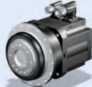
SMS PH(A) Planetary Geared Motor Acceleration torque PH(A): 27 – 7 500 Nm Backlash PH: \leq 3 - 4 arcmin Backlash PHA: \leq 1 - 2 arcmin Designed for high-performance servo drives
