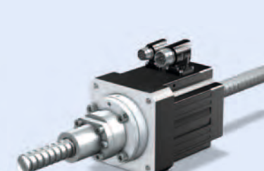
EZM Synchronous Servo Motor Screw nut driven by flanged hollow shaft Feed force at standstill: 923 – 26 138 N For any threaded screw length
