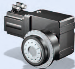
SMS PH(Q)K/PHKX Right-Angle Planetary Geared Motor Acceleration torque PHK: 89 – 7 500 Nm Acceleration torque PHQK: 123 – 22 000 Nm Acceleration torque PKX: 11 – 3 000 Nm Backlash PHK: \leq 3.5 - 4.5 arcmin Backlash PHQK: \leq 3.5 - 4 arcmin Backlash PHKX: \leq 3 - 6 arcmin Lots of variations with low backlash
