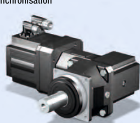
SMS PK/PKX Right-Angle Planetary Geared Motor Acceleration torque PK: 68 – 2 700 Nm Acceleration torque PKX: 11 – 3 000 Nm Backlash PK: \leq 3.5 - 5 arcmin Backlash PKX: \leq 4 - 8.5 arcmin Large ratio range
