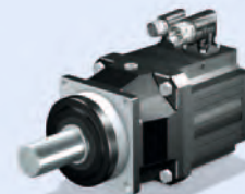
SMS P/PA Planetary Geared Motor Acceleration torque P: 11 – 3 000 Nm Acceleration torque PA: 20 – 1 600 Nm Backlash P: \leq 3 - 8 arcmin Backlash PA: \leq 1 - 3 arcmin Precision for positioning and synchronisation
