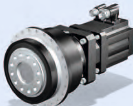
SMS PHQ(A) Planetary Geared Motor Acceleration torque PHQ: 72 – 22 000 Nm Acceleration torque PHQA: 72 – 10 000 Nm Backlash PHQ: \leq 3 arcmin Backlash PHQA: \leq 1 - 1.5 arcmin The ultimate servo quattro drive
