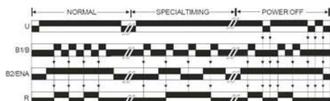
Tse – Toggle with starting contact and enable
