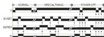
Fsc - Flip-Flop with starting contact and prior reset
